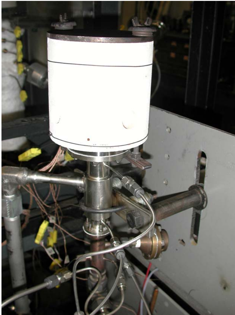
Figure 3: Photograph of 16 cm 3 jet-stirred reactor and SPP used by Edmonds [10]. SPP modified by Edmonds from original by J.C.Y. Lee [9].
